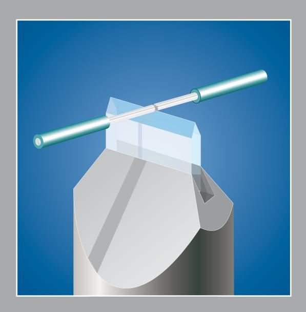
Diamond cleavers for fibre optic scoring
